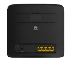
Huawei E5186 is the latest 4G LTE WiFi router with LTE Category 6. With the Carrier Aggregation technology, the Huawei E5186 could support peak download speed to 300Mbps and upload speed to 50Mbps. Up to 64 wireless users could access internet through Huawei E5186.
